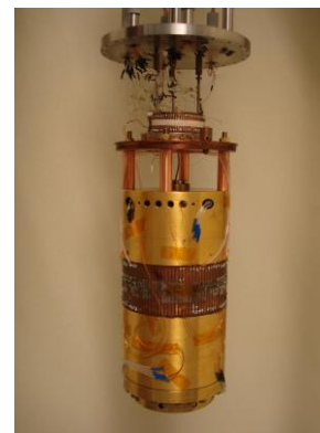
Fig. 2 Interpolating constant volume gas thermometer.
