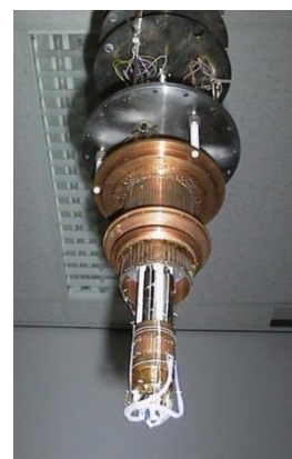
Fig. 1 Experimental set-up of the 4 He interpolating constant volume gas thermometer
