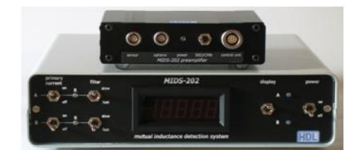
Fig. 10 Detection electronics to measure simultaneously SRD and CMN sensor signals.
