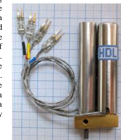
Fig. 9 Combined SRD and CMN sensor block.
