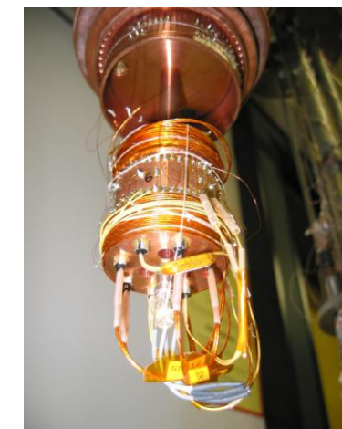
Fig. 7 Comparator block for the calibration of customers' thermometers.
