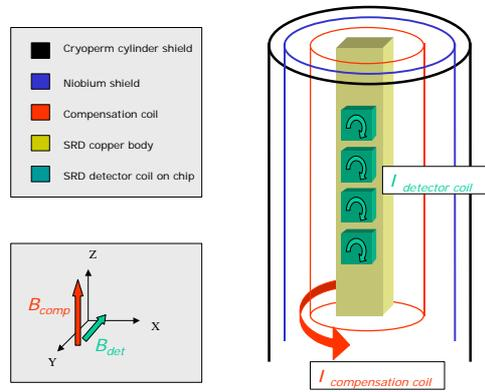
**Figure 3:** Shielding and field configurations of the SRD1000.
