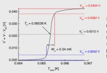
Example of a calibrated reference point at 65mK (superconductive transition of an  $Ir_{92}$ Rh<sub>08</sub> sample); the calibration parameters of the transition are indicated
