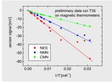
Preliminary results of measurements on the magnetic signal of some paramagnetic salts versus 1/T (the sensor signal is proportional to the susceptibility of the material)
