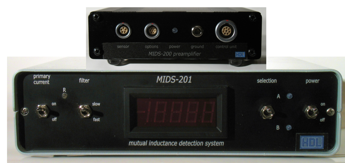
Figure 2. MIDS-201 (1-channel) detection electronics; the MIDS-202 is a version for independent and simultaneous 2-channel measurements.
