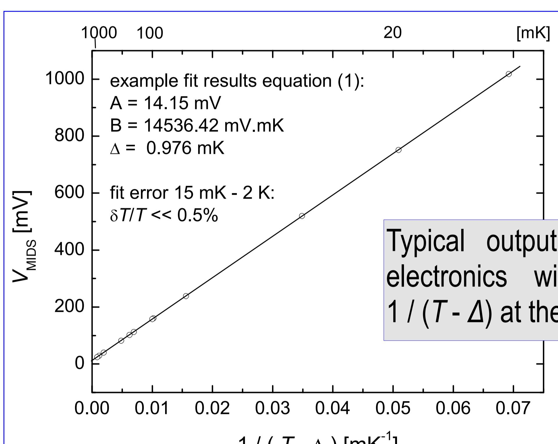
Typical output voltage of the MIDS20x electronics with CMN1000 sensor versus  $1 / (T - \Delta)$  at the SRD1000 reference points.
