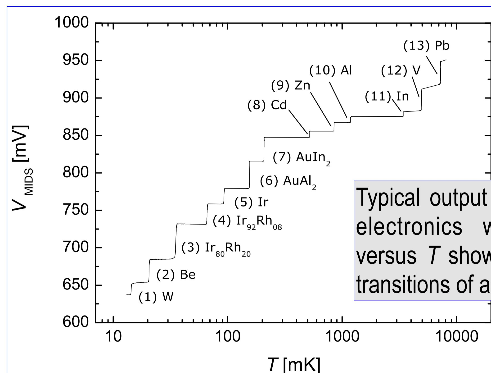
Typical output voltage of the MIDS20x electronics with SRD1000 sensor versus  $T$  showing the superconductive transitions of a 13-point sensor.
